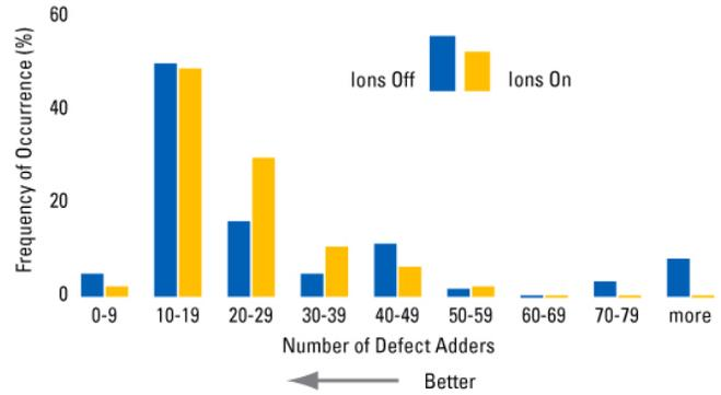
Figure 4. PVD tool results showing the number of particles before ionization and after ionization
