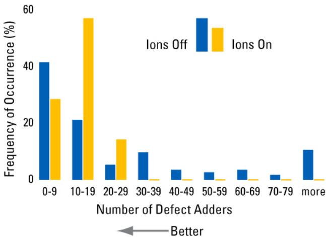
Figure 3. XRF tool results showing the number of particles before ionization and after ionization
