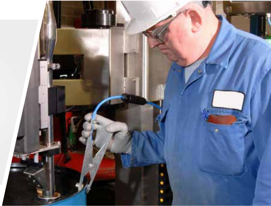
Medium and Large Heavy Duty Clamp/s with Quick Connect and optional lengths of Hytrel coated 2 core cable included
